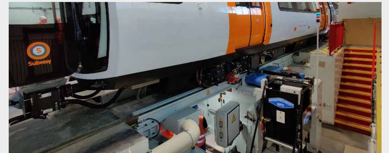
Wheel lathe fully operational and supporting future wheelset strategy.
