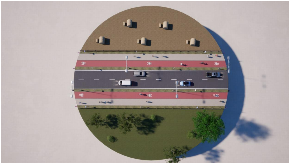
Example of a Primary Fully Segregated Unidirectional Cycle Route in a Rural Environment (Source: Sweco UK)
