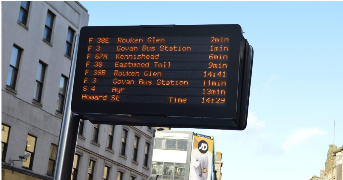
Figure 8: Example RTPI display unit
